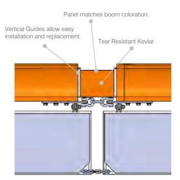
**TUFFBOOM** Deflector Panels prevent smaller surface debris from passing between boom sections. These versatile panels are especially favored for use near fish ladders and collection systems where even very small floatable debris can create large problems.
